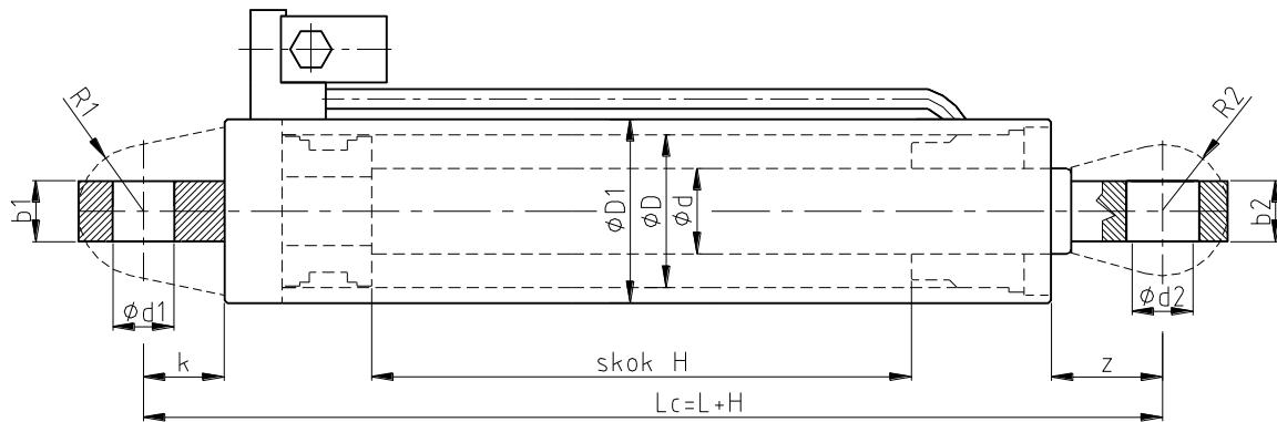
Example of hydraulic cylinder marking: **WHZz 1– 100x56x200 / 530x0 – 3 –B**
