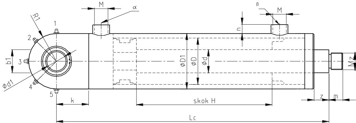
hydraulic cylinder marking: **WHC 2 - ..... x..... x..... x / .....x - ..... - ..... A,B,C**
