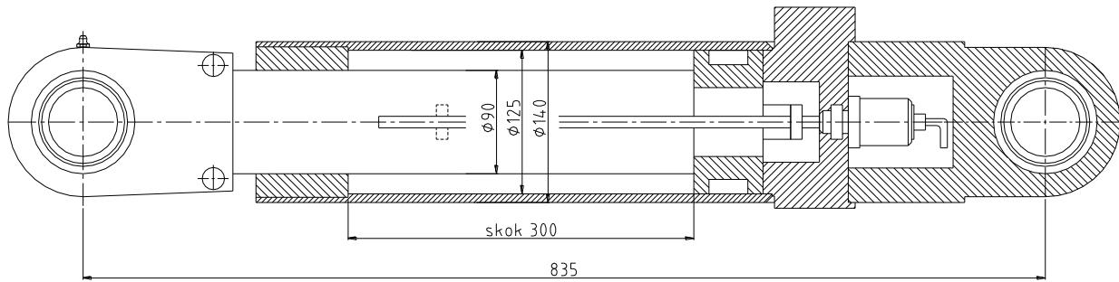
Picture 1 – Hydraulic cylinders with stroke length measurement.
