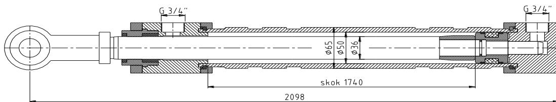
Picture 3 – Modular hydraulic cylinder with GIKFR end.
