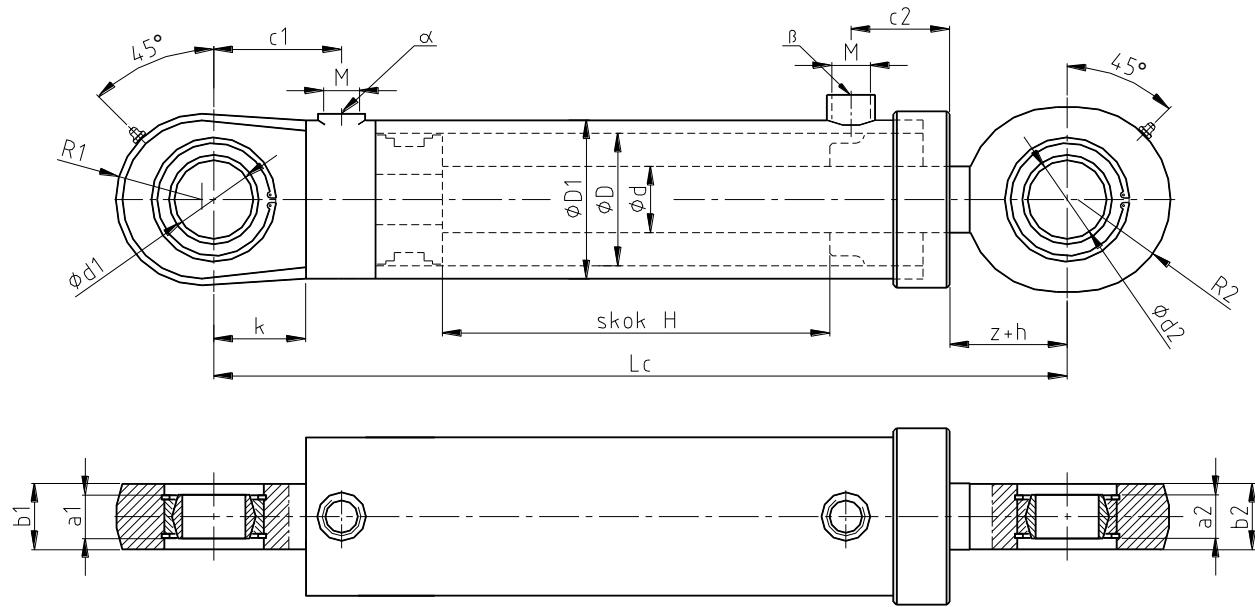
Example of hydraulic cylinder marking: **WHC 3 – 100x50x560 / 1024x0 - 0/0 - B**
