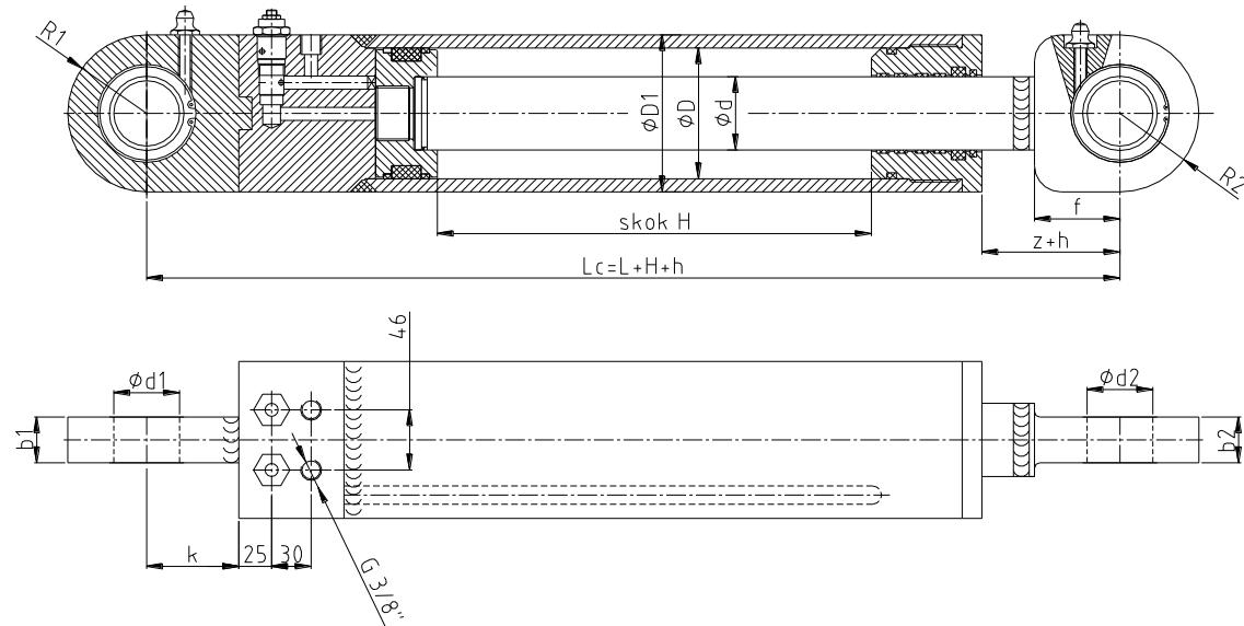
Example of hydraulic cylinder marking: **WHZn 2– 95x56x300 / 710x13-1-B**
