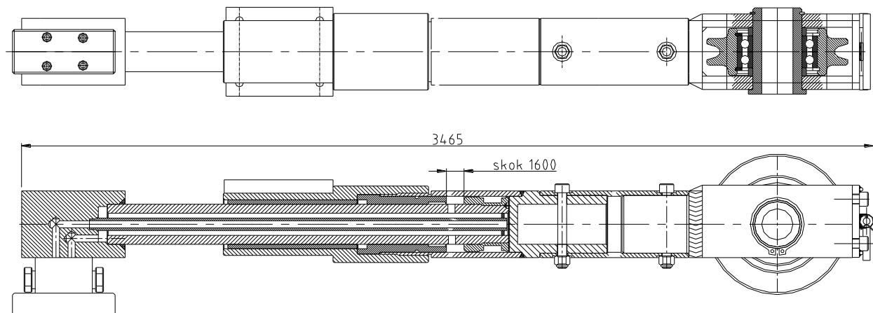
Picture 6 – Hydraulic cylinder fed by piston rod
