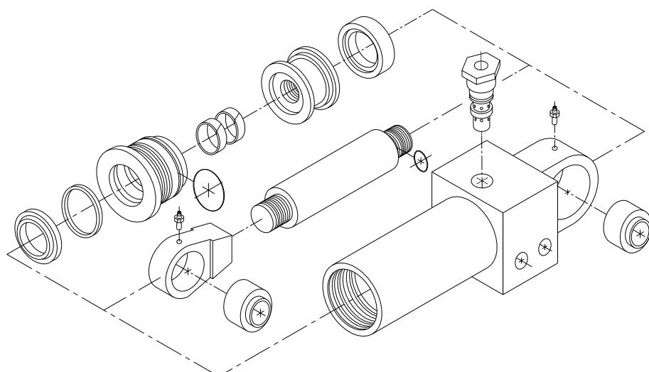
Picture 8 – Hydraulic cylinder with cartridge valve
