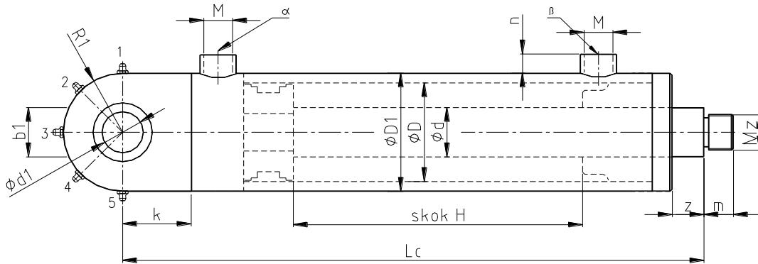
hydraulic cylinder marking: **WHC 1 - ..... x..... x..... x / .....x - ..... - .....**
