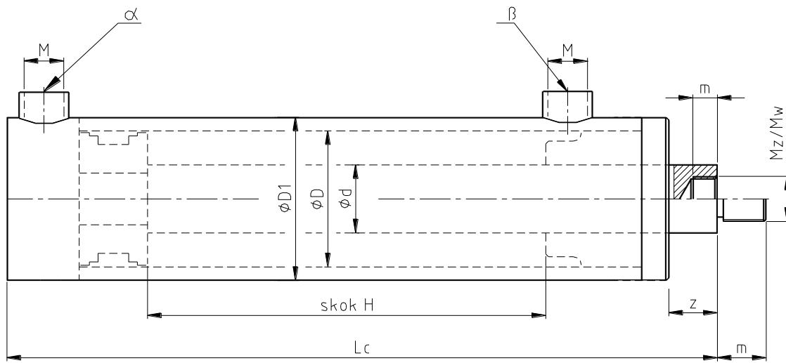
Example of hydraulic cylinder marking: **WHC 7A-25x16x100 / 208x10-0/0 -B**
